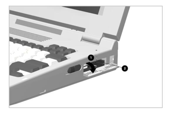
Figure 5-14. Removing a PC Card
